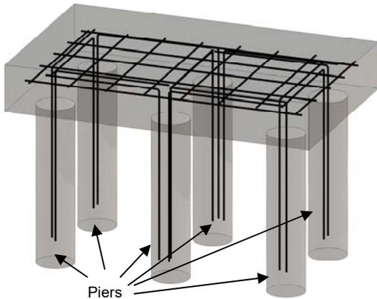
Figure 4. Footing with Piers - Cutaway View
